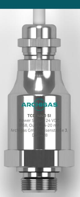
The compact and robust TCD3000 SI (Screw-In) transmitter is ideally suited for precise, fast, and sensitive measurement of (quasi-)binary gas mixtures. The measurement is based on the principle of thermal conductivity. This technology is ideal for measuring gases with significantly different thermal conductivities, such as H2 and O2.
